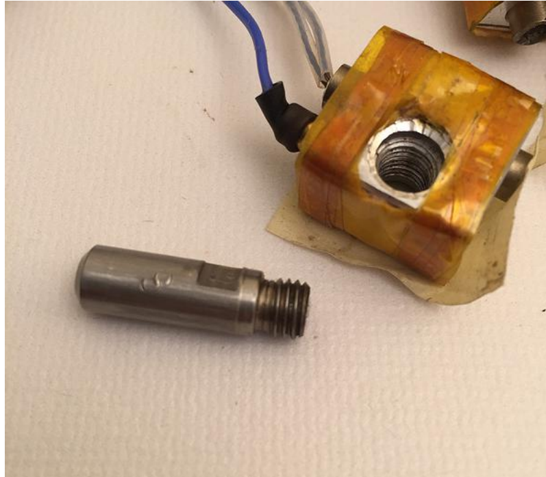
17. Unscrew and remove thermal tube from left and right heater block.
