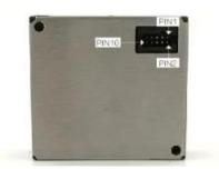
PIN1 VCC power supply positive (+5V)
