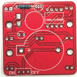
A red PCB with various components. A 100 Ohm resistor is being soldered to the board. The board has a red circular marking and a '+' sign. The text 'ON' and 'OFF' is visible at the bottom. | <p>Der 100 Ohm Widerstand wird eingelötet</p> |
