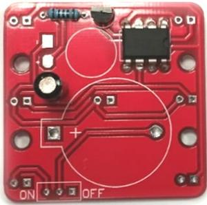
A red PCB with various components. A small black tilt sensor is being soldered to the board. The board has a white circle and a '+' sign. Labels 'ON' and 'OFF' are visible at the bottom. | <p>Der Neigungssensor wird eingelötet.</p> <p>Die Ausrichtung ist dabei egal.</p> |
