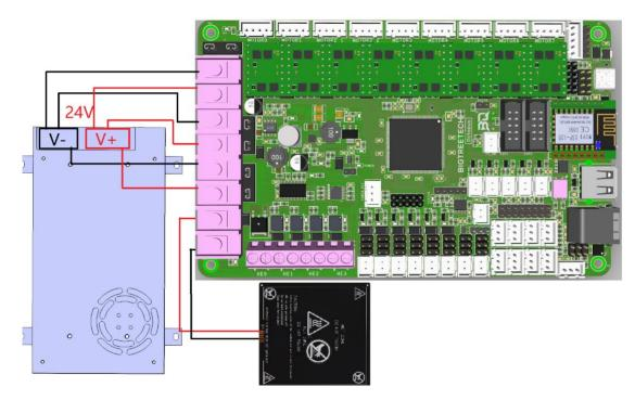
Note: DO NOT alter the board wiring with the power on and be sure to get the polarity correct, otherwise you can cause damage to the motherboard.
