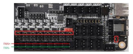
Note: Since the jumpers carry a voltage rail directly from one of the regulators or from the input, if you short the jumpers in any way other than the shown connections, you will likely cause damage to the motherboard. When connecting the fan, make sure that you connect the positive terminal to the positive output as shown in the images.
