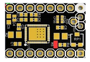
(1)Welding resistance at R5 position to make the driver STP/DIR working mode;(2)Work mode selection: SDI (CFG1), SCK (CFG2)
