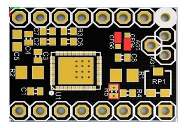
Remove the resistance at the R5 position so that the driver is in SPI working mode.
