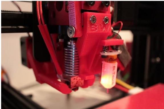
Heater cooler with right hand side mounting of the original 40 mm cooler fan. Can be used with or without a BL-Touch. Uses BL-Touch with the springs that come with them by standard since Nov-2016.
