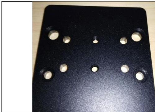
As of Apr-2017, The stock Z-wheel plates come with tapped M5 holes for the POM ACME nut screws. In order to lock the screws, you need a regular nut.
