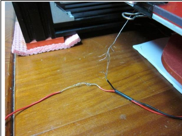
The pre-tinned stranded Copper wire **is not recommended** for use inside the drag-chain.
