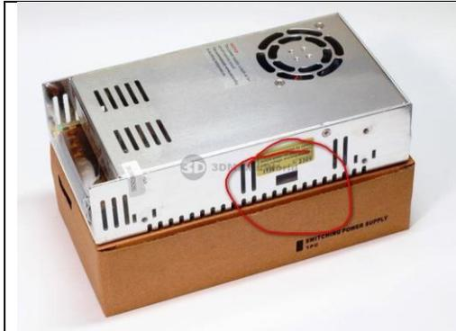
**Check the V<sub>AC</sub> selector switch.**
