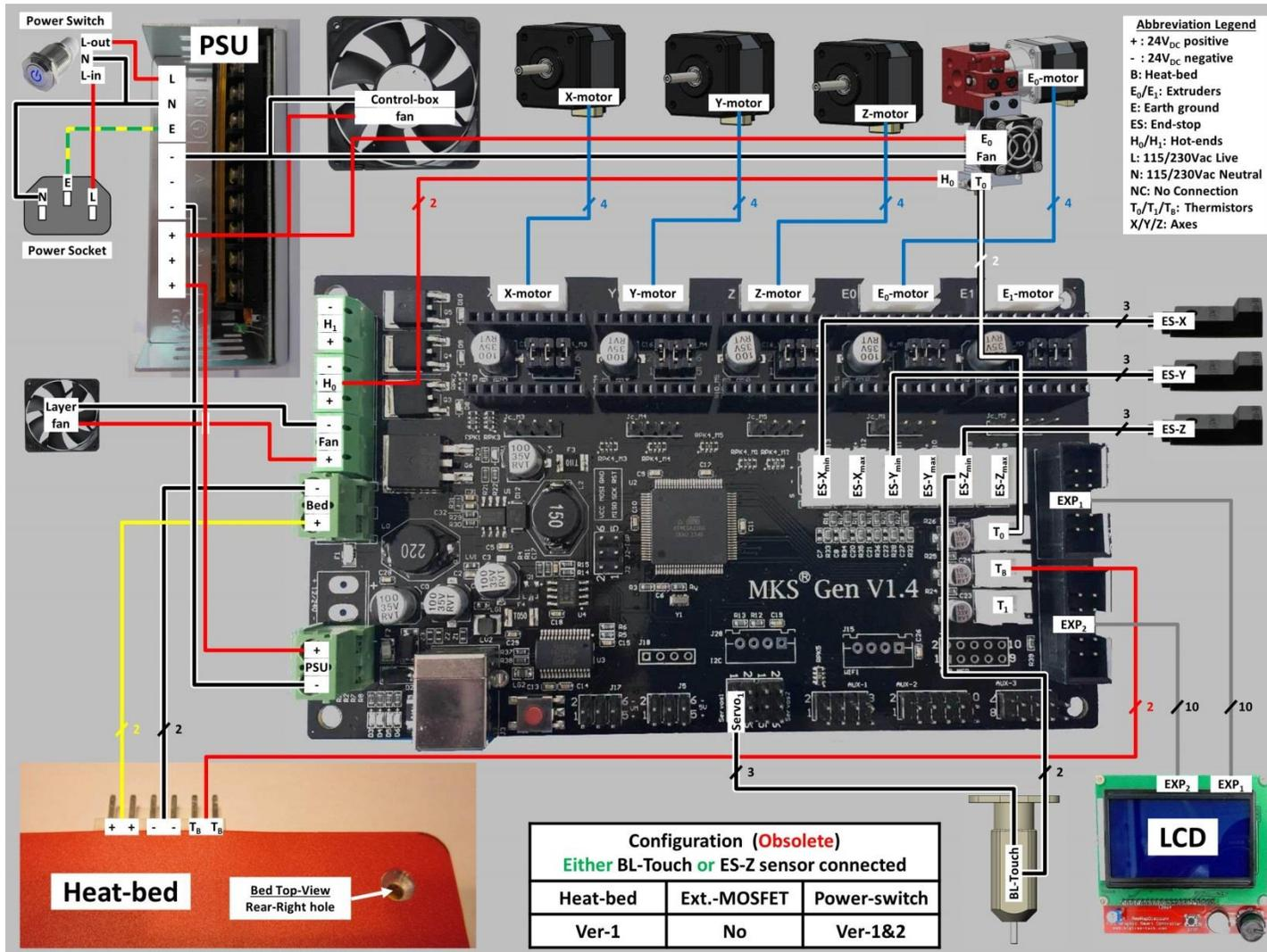
7.10.2 Heat-bed - V2; Power-switch - V1&V2
