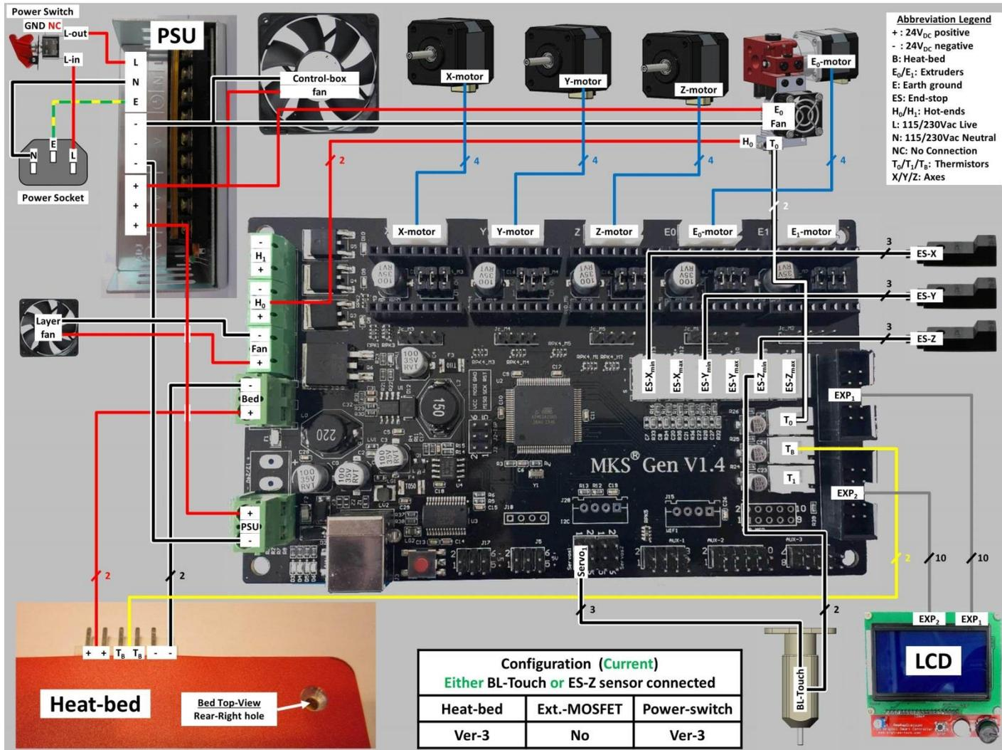
7.10.4 Heat-bed - V3; Power-switch - V3; with External MOSFET
