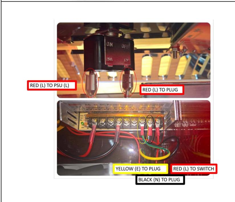
With the new supplied power switch from TEVO you need to route the 110/220 VAC wires as shown on the pictures.
