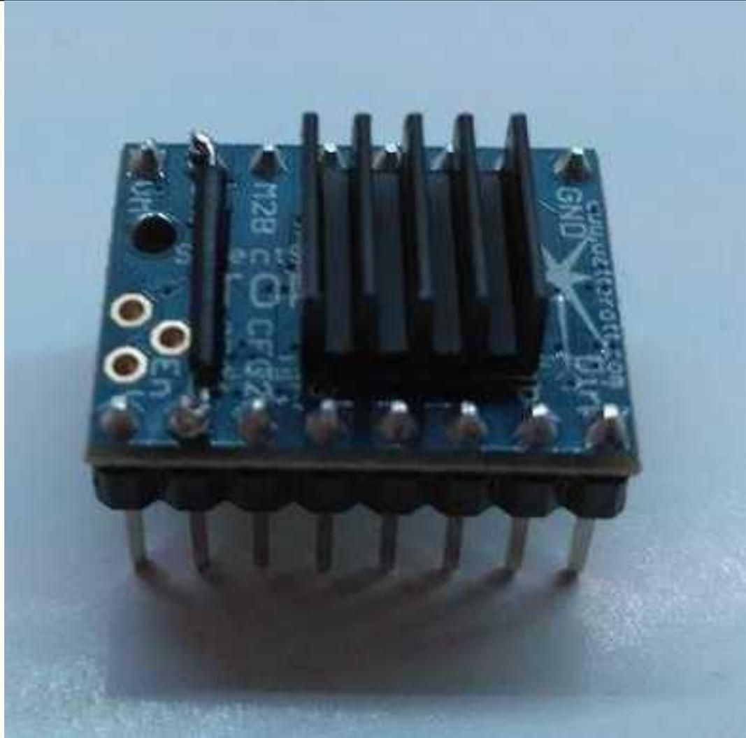
**Method-2 for connecting CFG1 to GND**
