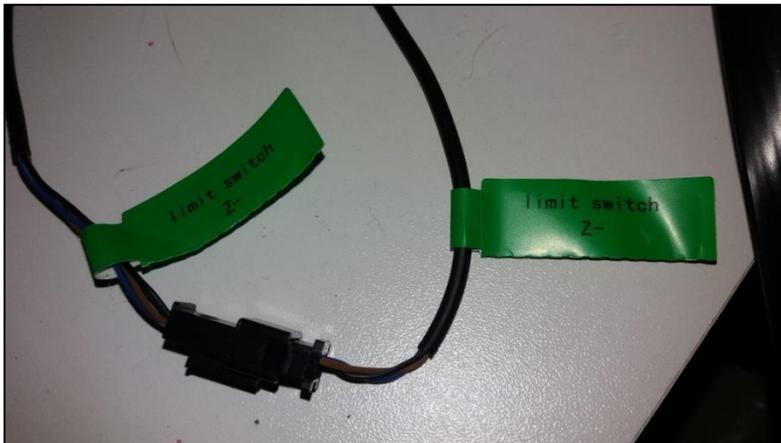
Connect the white/red cable coming from the BL-Touch 2 wire cable to the Limit switch Z-.
