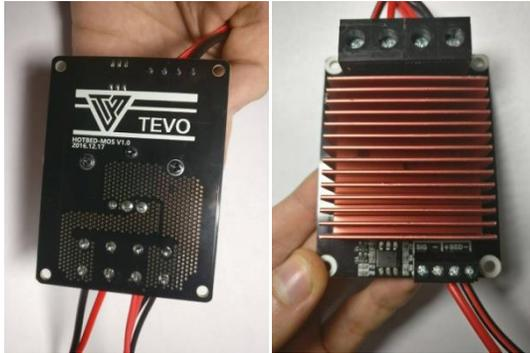
Due to the problems with the MKS GEN V1.4 boards TEVO designed a high power **EHD** (External **H**eat-bed **D**river) board. From 13-Jan-2017 all warranty MKS GEN V1.3 and V 1.4 replacements boards get this **EHD** standard shipped along with a new MKS GEN V1.4 main board.
