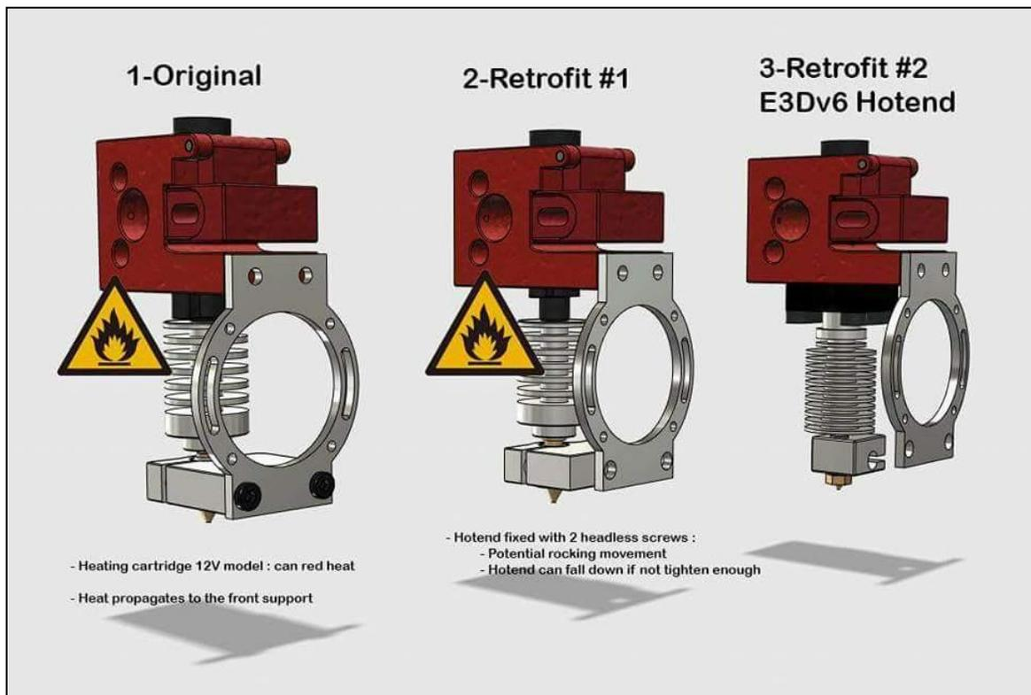
As it comes from TEVO, the nozzle sits against the heat-block, not the heat-break, thus may cause leakage of filament above the heat-block.
