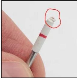
Assemble the BLT again and make sure the top of the hexagon screw is flush with the top of the BLT mounting.
