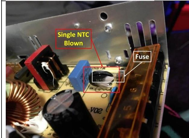
**Check the NTC resistor.**
