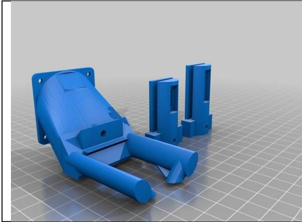
Filament cooler for E3D V6 with regular or Volcano heater Block. Uses a 40 mm cooler fan. This is a layer fan duct which cools the object, not the hot-end's heat-sink.
