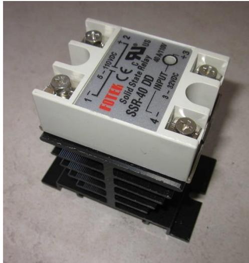
You may accomplish the same heat-bed offload functionality, by using an industry standard SSR. This is an electronic SPST (Single Pole Single Throw) switch, which is connected in series on the +24V line, between the PSU and the heat-bed, and is controlled by the “Bed” output of the MKS-Gen controller.
