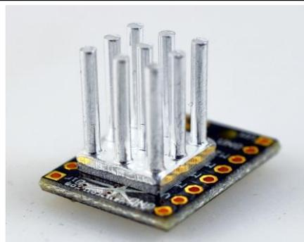
When using the **TMC2100 Black-PCB 3.3V-5V version**, you'll probably need these heatsinks in order to get the max torque out of the stock motors, without entering into the thermal protection zone.
