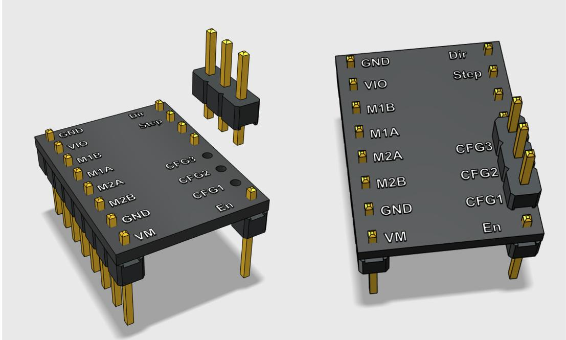
Below left picture: "Standard" driver stick. Right picture shows CFG pins facing up.
