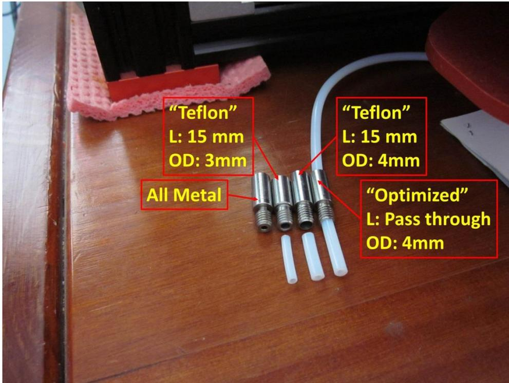
1) The “All metal” type is **NOT** recommended as in most clones the 2 mm bore is not concentric with the nozzle bore. The resultant “step” at the interface, between the nozzle & the heat-break, will cause a clog within 5 minutes to few hours.
