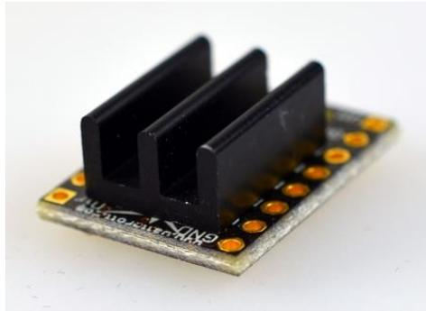
When using the **TMC2100-5V Blue-PCB 5V-only version**, the power dissipation is lower, therefore these heatsinks suffice in order to get the max torque out of the stock motors, without entering into the thermal protection zone.
