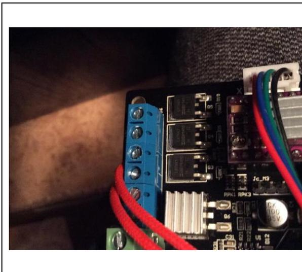
Due to failing Q6 power MOSFETs which control the heat-bed (reason is probably over-stressing of Q6), then from 18-Dec-2016 TEVO QC (Quality Control) checks all boards (they say) and adds a small heat-sink on the heat-bed MOSFET. The heat-sink will not do any work but it lets you know you have a factory QC tested board.
