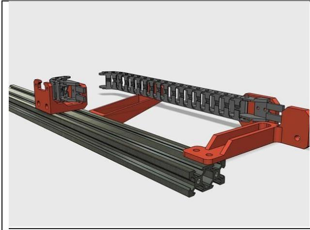
A side-mounted Drag-Chain that enables you to squeeze the max height on your Z-travel.
