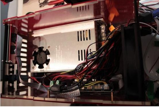
When you are printing direct from a SD (Secure Digital) card and you have random problems during printing like reverse extruding, motors stopping, shifting layers and other unexpected movements make sure the grey LCD (Liquid Crystal Display) cables are not running over the power supply. If you use a SD card for printing the data from the card to the main board gets corrupted due to electronic signals from the power supply. Reroute the cables away from the power supply like the picture shows.
