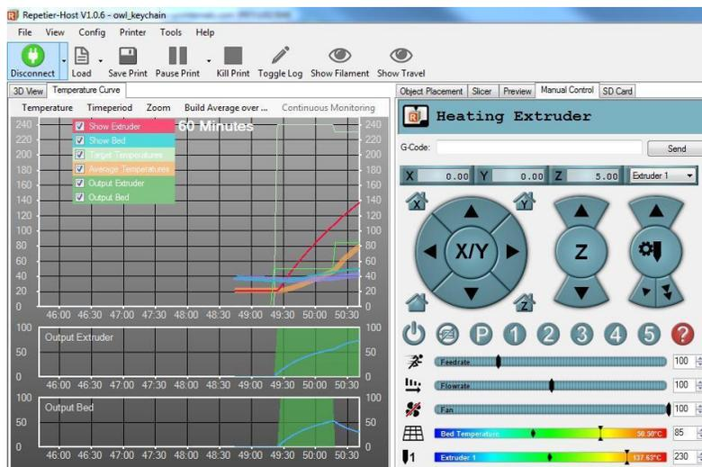
In the Manual Control section home first X/Y and Z in this order and if it is not the case move the nozzle to the center of the heat-bed with the cursor control.
