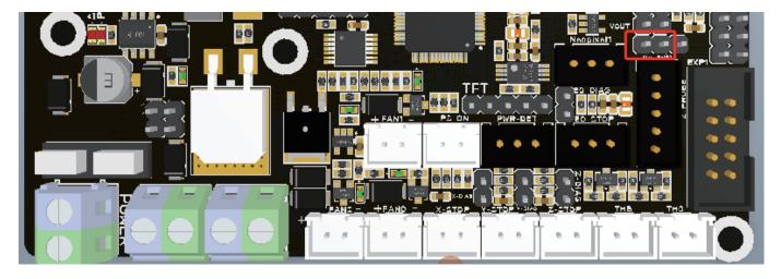
2. To use an external BIGTREETECH DCDC5V V1.0 module, short the pins shown in the above image using a jumper.
