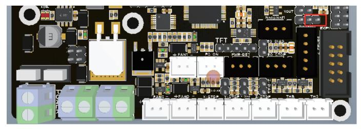
1. To use the onboard 5V PSU, short the pins shown in the above image using a jumper.
