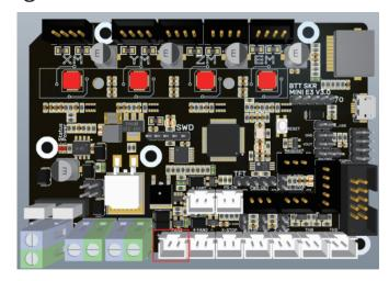
Connect the fan by FAN2 to realize the whole machine cooling.
