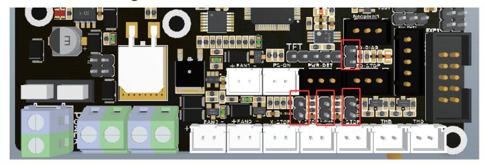
As shown, connect the corresponding axes with the jump caps to choose Sensorless homing function
