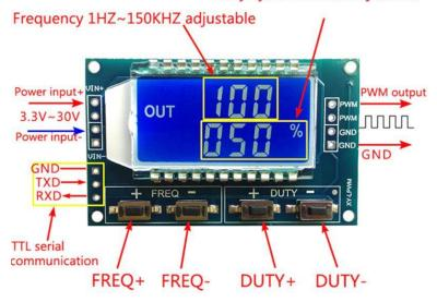
Output PWM amplitude=Input voltage
