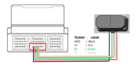
Figure 1 Schematic Diagram of Connecting TFmini-Plus with TELEM 2 Interface (Serial Port 2) of CUAV V5
