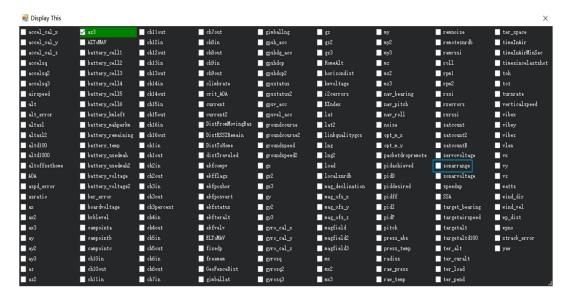
The altitude distance from the LiDAR will be displayed in Sonar Range (meters), see the following picture:
