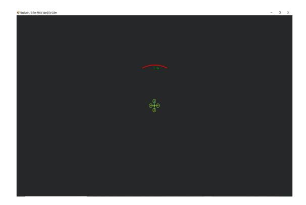
The number in green color means the distance from LiDAR in obstacle avoidance mode (it doesn't mean the real time distance from LiDAR and will not be influenced in Mission Planner. The mission planner version at the time of writing this tutorial was v1.3.69.
