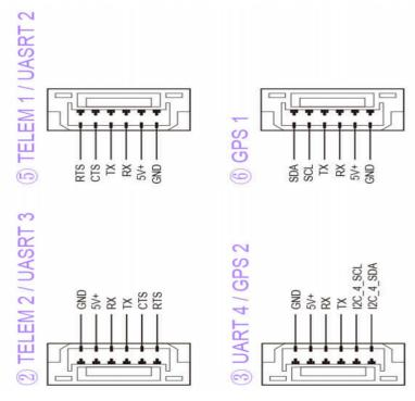
Figure 2 Pinout description of available serial ports on CUAV V5
