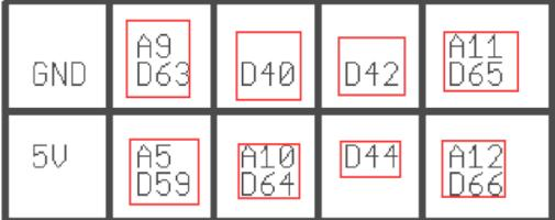
As shown in the IO port diagram above, when writing firmware, you can choose to write A+ number or directly write A number, such as A9
