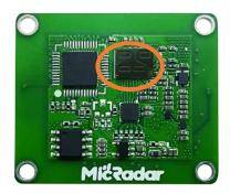
The part enclosed in yellow is the radar antenna
