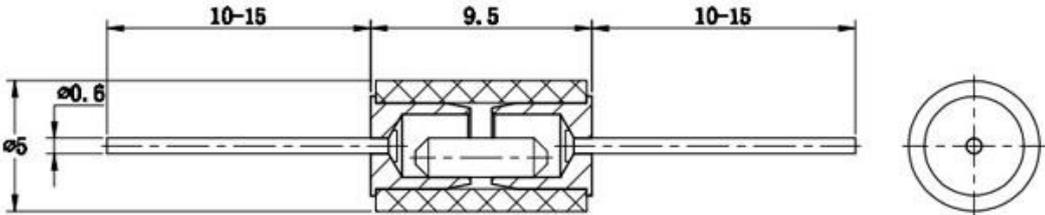
Omni-sensing various directions of vibration
