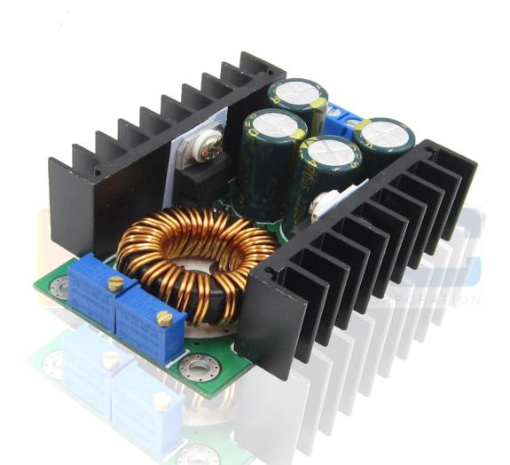
It is a buck converter module consist of two XLSEMI XL4016 regulators connected to two heatsinks, four 470µf capacitors and two potentiometers for current and volt adjustment.
