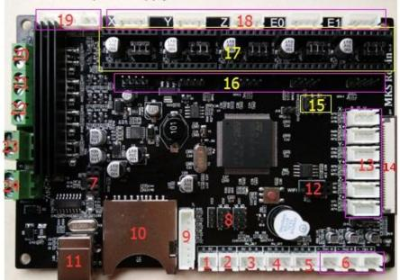
1,2. 5V output 3.MKS DET(UPS) 4.MKS PWC 6.E0,E1 thermistor 7.MKS DET 5.filament interrupt detection module 8.expansion PIN for steering engine,ect 9.SD expander 10.SD 11.USB 12.WIFI 13.endstop 14.TFT screen
