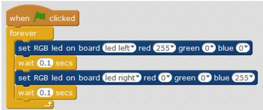
On the board, these two LED lights are individually controlled, keeping constantly their current state (for instance, if you only turn the left LED light on, then its state will remain lighting up). At this very time, if turn on the right LED light, the program won't change the state of the left LED, then you will see both LED lighting up, without flickering effect.
