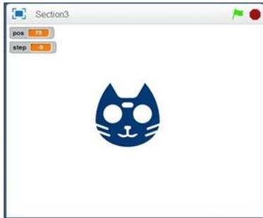
Click the small green flag to start the program, and press on the infrared remote control the key number 1. You should see that “step” value is 5, so “pos” value continues to increase y step value, making the robot to look on his left. Release the button, the value won't change, and the robot also stops turning.
