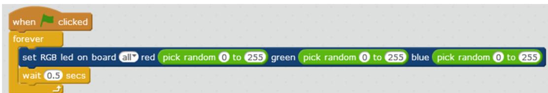
Figure 34 Automatically Display RGB LED every 0.5s
