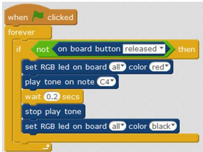
Figure 60 NOT Logic Operators Script
