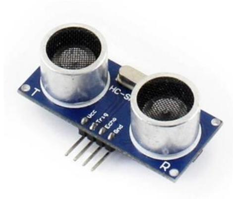
Figure 79 Ultrasonic Sensor
