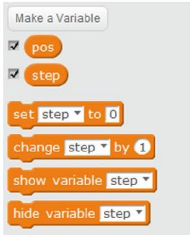
: Here, we first set both "pos" and "step" variables. Pos value represents the current position of the steering gear. Step represents the angle of each rotation. A positive number means a left turn. And a negative number means a right turn.
