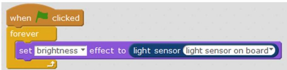
Figure 66 Using The Light Sensor Script
