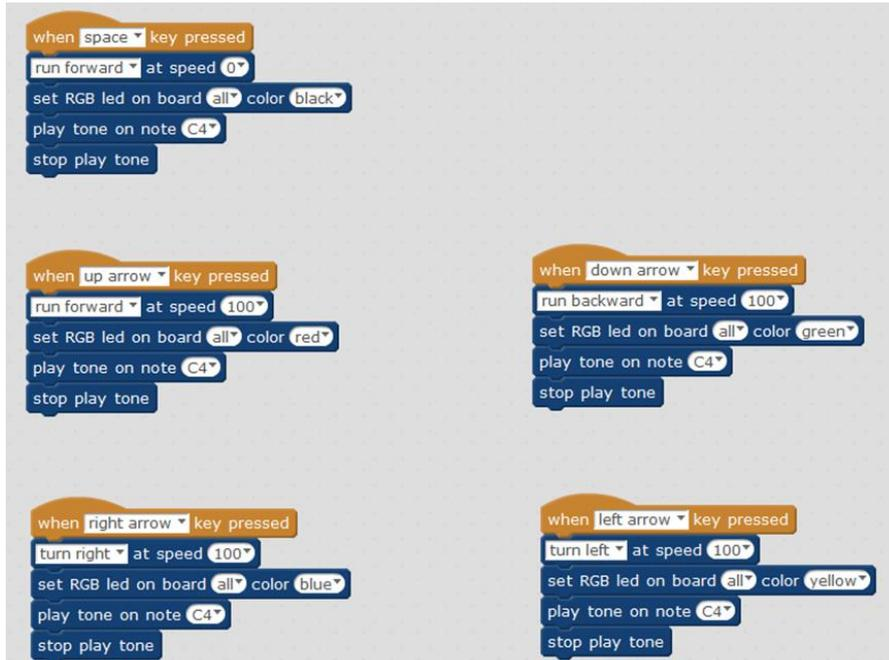
Figure 44 Control KitiBot by Keyboard Script
