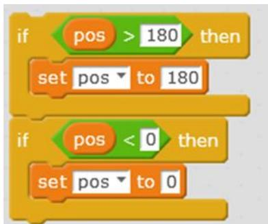
The two “conditional blocks” are to determine if the angle is greater than 180 degrees or less than 0 degrees. If it’s about 180 degrees, the angle is set to 180 degrees, and if it’s less than 0 degrees, it always will be set to 0 degrees. Because of this, the robot head can only rotate within an angle range, which is from 0 to 180 degrees.
