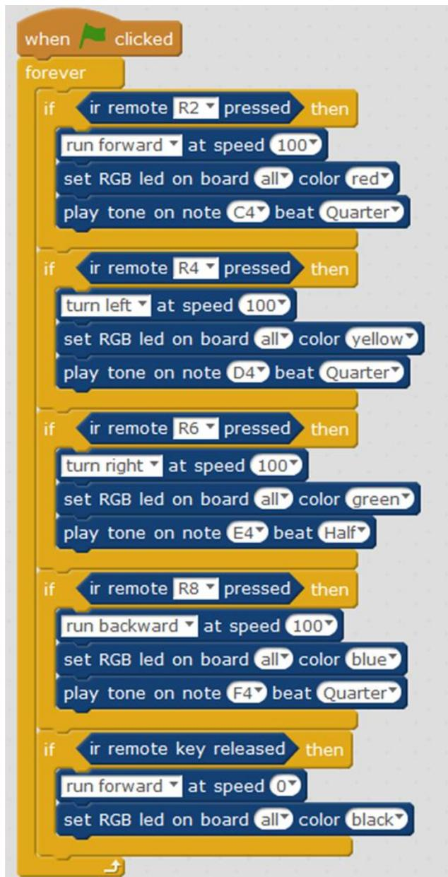
Figure 72 Key Status of IR Remote Controller Script
