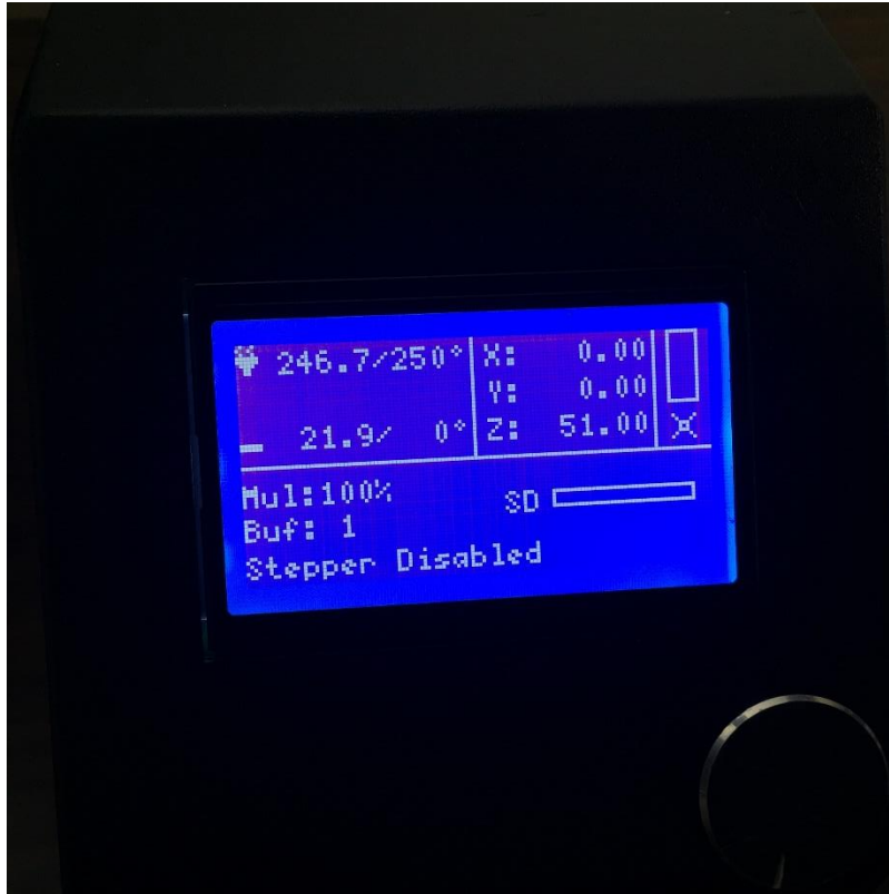
19. Preheat the nozzle to 250C.
