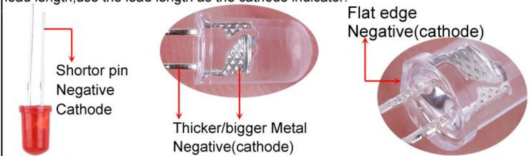
Step 12: Install 81pcs 5mm Red LED at L1-L81.
