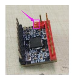
Note: This function pin needs to be trimmed only when the blocking detection function is not used.
