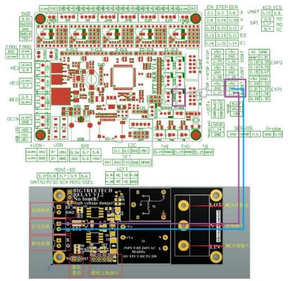
6. The connection of SKR V1.4 and Resume Printing While Power Off Module (UPS  $24V\ V1.0$ ) :
