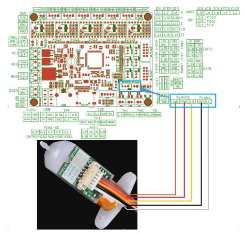
5. The connection of SKR V1. 4  $\,$  and Automatic Shutdown After Printing Module (Relay V1.2) :
