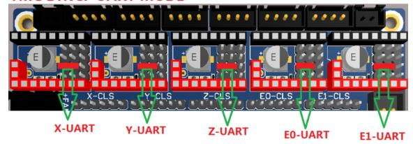
Note: When using the TMC2209, if you don't use the stallguard function, you need to cut off the DIAG pin on the driver so that the mechanical switch can work normally. The operation method is as shown below:
