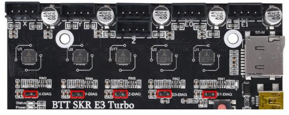
As shown in the figure, the Sensorless homing function can be used to connect the corresponding axis with the jumper cap.
