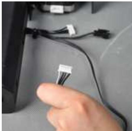
17. Connect end stop switch to socket switch directly onto its position. For some printer you may need to install the switch onto the side wall.
