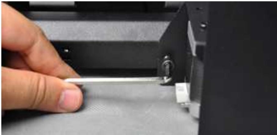
13. Turn printer aside, Lock extra 2 bolts inside base 14. Lock the left motor cable
