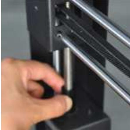
11. Insert the Base into the tower and match the bolt hole.
