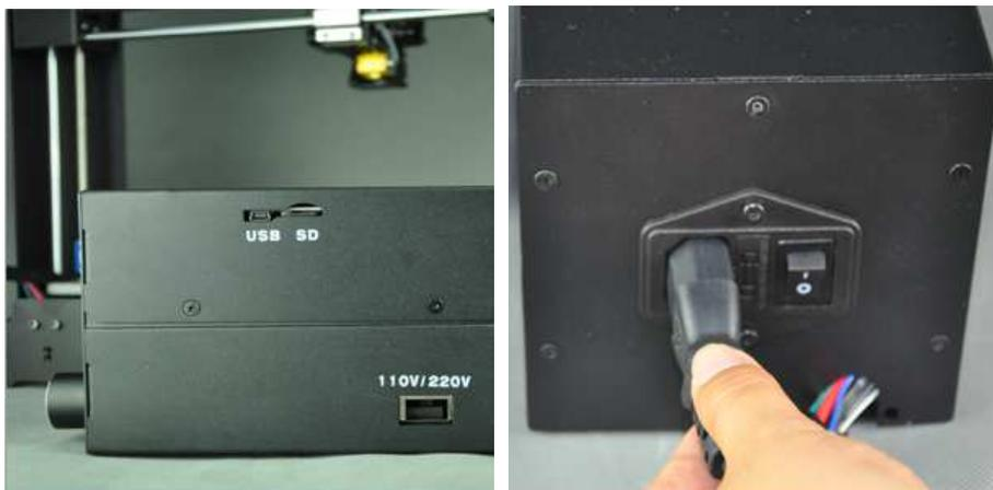
To protect the motor cable from damage during shipping, we have unplugged the Z axis and X axis motor cable connector. You need to insert the connector into the socket when you start. The longest cable is for X axis. And the other 2 male connectors quite near the female connector are for Z axis motor. Just insert them.
