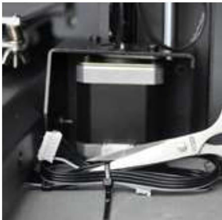
16. Short cable for Z; Long for X, black for end stop switch
