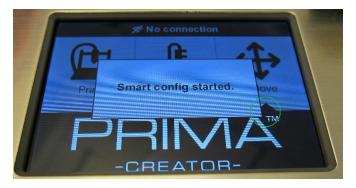
When the application is connected to your Wi-Fi, turn on the printer. Navigate the "arrow "so that it is under "Move". Push down the button. You will see the text "smart config started". It can take up to one 1 minute for the config to be done.
