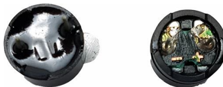
Links aktiver Buzzer; Rechts passiver Buzzer
