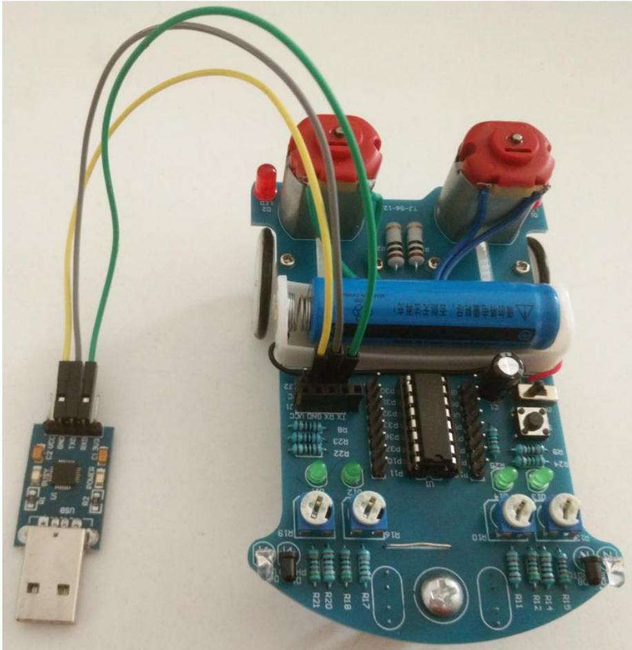
Serial port module and D2-6 trolley connection
