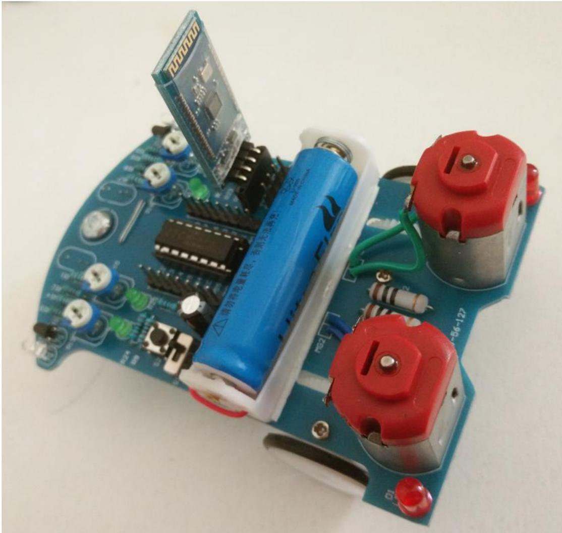
When the Bluetooth module is powered on, if there is no connection with the host computer, the indicator on the module is flashing. When the connection is connected, the indicator on the module is on.
